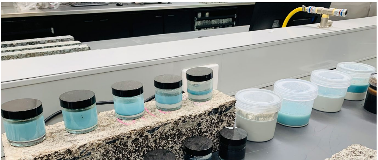
Paintback testing taking place in the Australian Research Road Board's laboratory.
